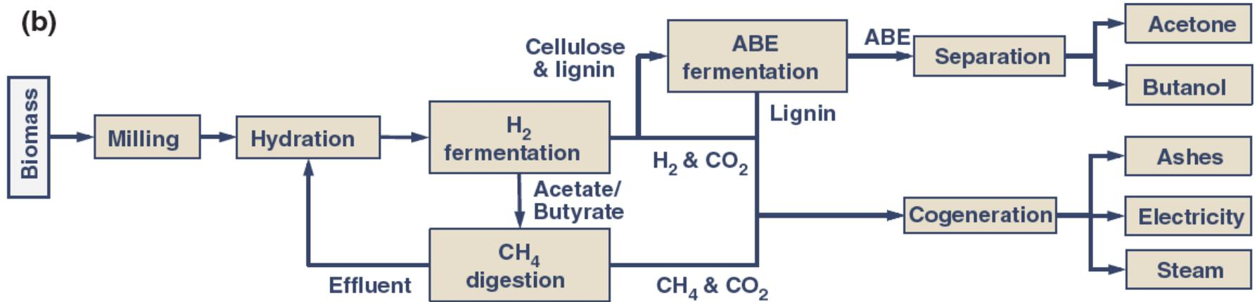
Figure 1. a) Reaction scheme for the biorefinery based on mixed cultures indicating the material flow. b) Process block diagram.
