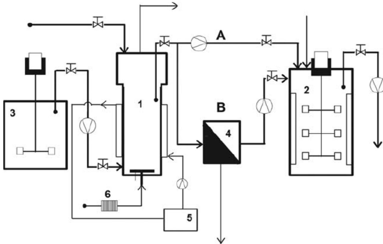
**Figure 1.** Continuous coupled enzyme production and saccharification system. (1) Bubble column (CMCase and xylanase producing reactor); (2) stirred tank (RENZ); (3) sterile reservoir; (4) centrifuge; (5) warm bath, and (6) air filter.
