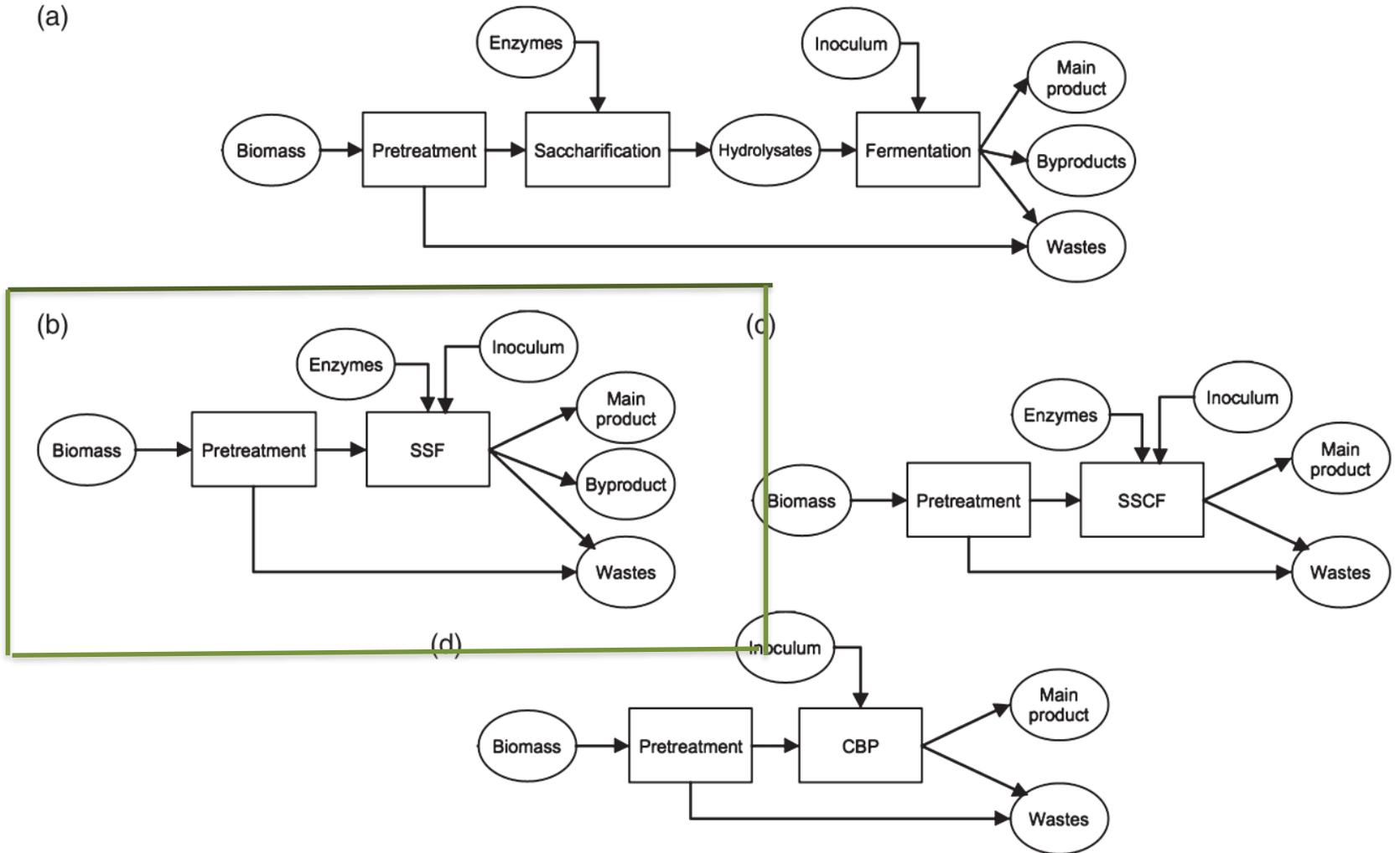
**Figure 2.** Saccharification and fermentation of biomass: (a) conventional; (b) SSF; and (c) SSCF and CBP.
