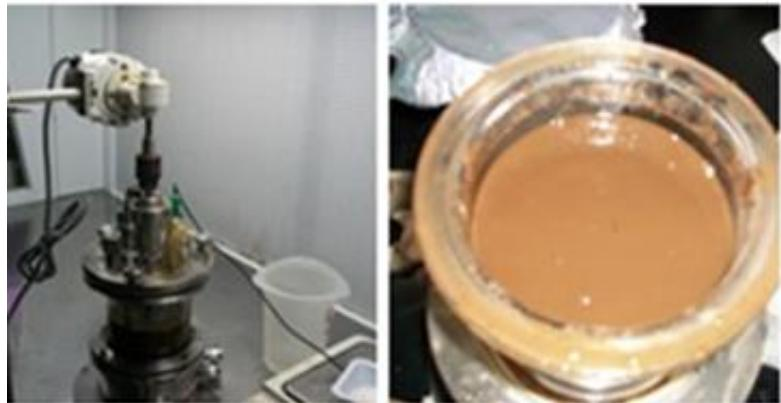
Most of the Xylose & Glucose are released from the pretreated corn stover above 1% H<sub>2</sub>SO<sub>4</sub> in 12 – 24 h
